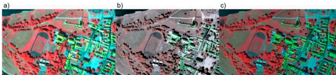
Figure 5. Examples of mosaics produced using images acquired in 2015: (a) HSI image, pixel size 0.7 m, R—Band 15 (WL852.71 nm), FWHM 14, G—Band 9 (WL703.02 nm), FWHM 9, B—Band 3 (WL553.46 nm), FWHM 9; (b) CIR image, pixel size 0.2 m, R—NIR band (~750–940 nm), G—Red band (~560–760 nm), B—Green band (~470–630 nm); and (c) panchromatically pan-sharpened HSI image using the CIR mosaic as a panchromatic image.
