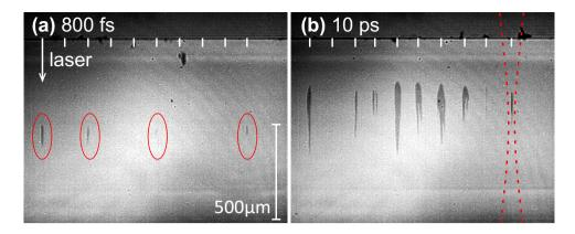
**Fig. 2** Typical examples of the induced modifications in silicon using pulse durations of 800 fs (a) and 10 ps (b). Focus position is located at 500  $\mu$ m below the surface. The red dashed line schematically illustrates the beam caustic for an undisturbed beam. The other processing
