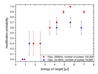
Fig. 3 Modification probability for different repetition rates and number of shots at 10 ps
