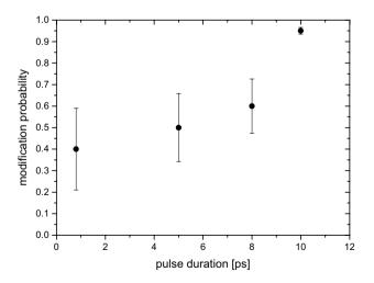
Fig. 4 Modification probability for 6.6  $\mu J$  at 30 kHz (15,000 shots) for different pulse durations
