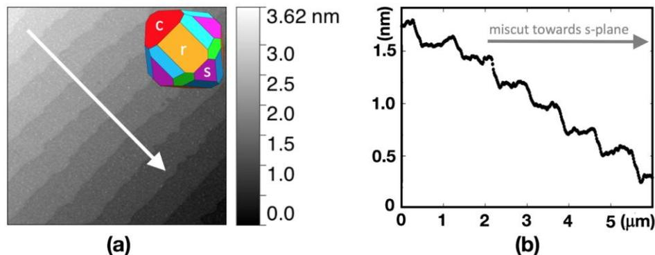
**Figure 8:** (a) AFM image ( $7 \mu\text{m} \times 7 \mu\text{m}$ ) of the sapphire substrate with the ECS sapphire inserted at the top right, and positioned crystallographically parallel to the substrate; (b) step profile taken along the white arrow in (a) showing that the surface is miscut towards the s-plane (purple facet of the ECS).
