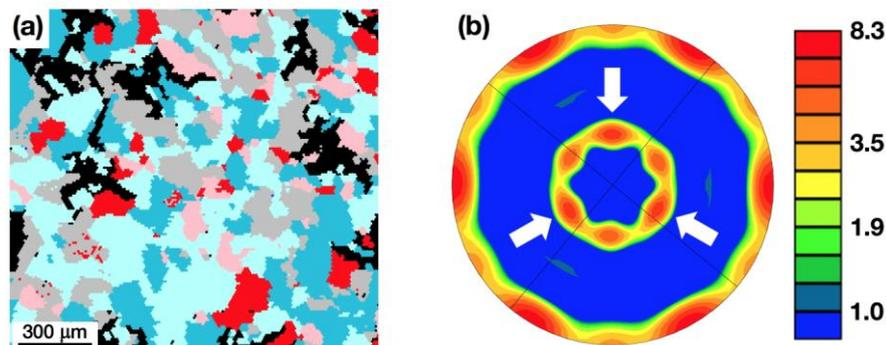
**Figure 7:** Data from a thick Cu film annealed on the r-plane of sapphire: (a) 1.5 mm x 1.4 mm EBSD map scanned with a 10  $\mu\text{m}$  step, where the grains are colored according to their orientation relationship on the sapphire (see text); (b)  $\{110\}$  PF of the Cu grains, showing the distribution of the  $\{110\}$  poles (units are in MRD); arrows mark the poles of the preferred OR (corresponding to OR1r/t).
