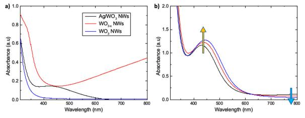
**Figure 2.** UV-visible absorption spectra for the three forms of tungsten oxide NWs (a) and evolution of the absorption spectra with silver growth for Ag/WO<sub>3</sub> NWs (b).
