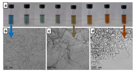
**Figure 1.** (a) Control of the silver island density from WO<sub>3-x</sub> NWs (**left**) to Ag/WO<sub>3</sub> NWs (**right**) as a function of time. TEM images for WO<sub>3-x</sub> NWs (**b**), intermediate density of silver islands on NWs (**c**) and final Ag/WO<sub>3</sub> NWs (**d**).
