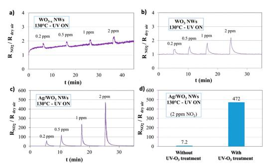
**Figure 3.** Sensor responses at 130 °C under UV illumination for WO<sub>3-x</sub> NWs (**a**), WO<sub>3</sub> NWs (**b**) and Ag/WO<sub>3</sub> NWs (**c**). Comparison of the sensor responses for Ag/WO<sub>3</sub> NWs with or without the UV-O<sub>3</sub> post-treatment (**d**).
