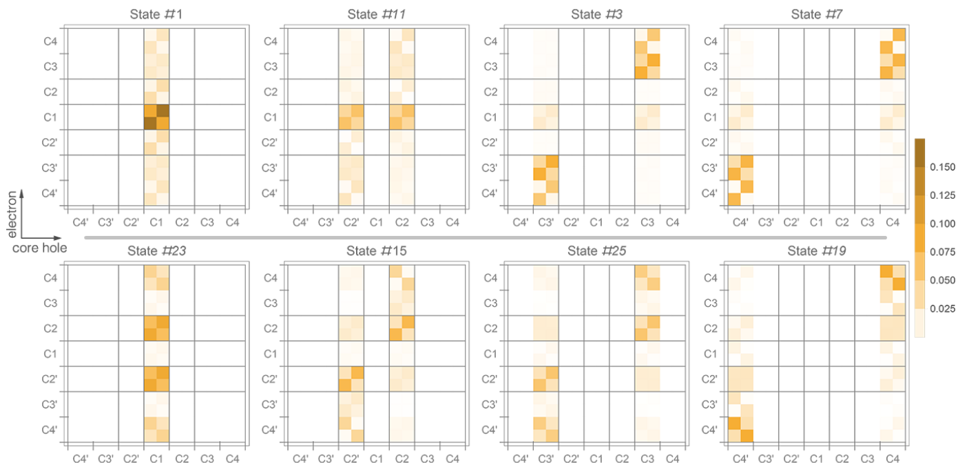
Figure 5. Electron-hole correlation plots of the \Omega_{AB} matrices for carbon K-edge states in the anthracene ( C_{14}H_{10} ) molecule. The upper graphics shows the first excited states for each different carbon site, representing the first excitation band in the spectra, whereas the lower graphics shows it for the second band.
