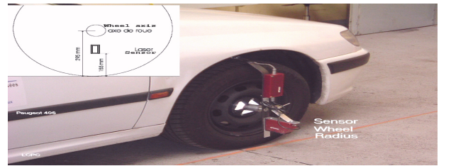
Fig. 5. Sensor for wheel radius measurement
