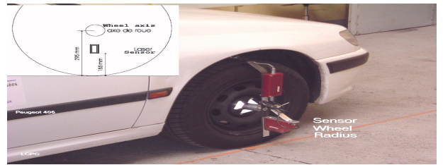
Fig. 5. Sensor for wheel radius measurement
