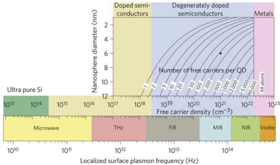
Fig. 7. Localized surface plasmon resonance (LSPR) frequency dependence on free carrier density and doping constraints @Nature (extracted with permission from ref 30 - <https://doi.org/10.1038/nmat3004>).
