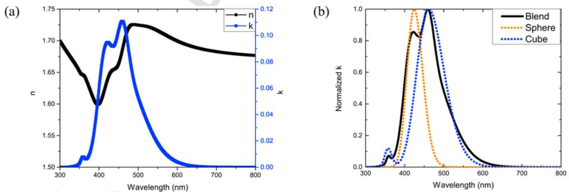
Fig. 15. (a) Complex refractive indices  $n$  and  $k$  of nanospheres and nanocubes blend in PVP and (b) the normalized extinction coefficient  $k$  compared to the one of nanospheres in PVP and nanocubes in PVP. @OSA (extracted with permission from Ref. [116]).
