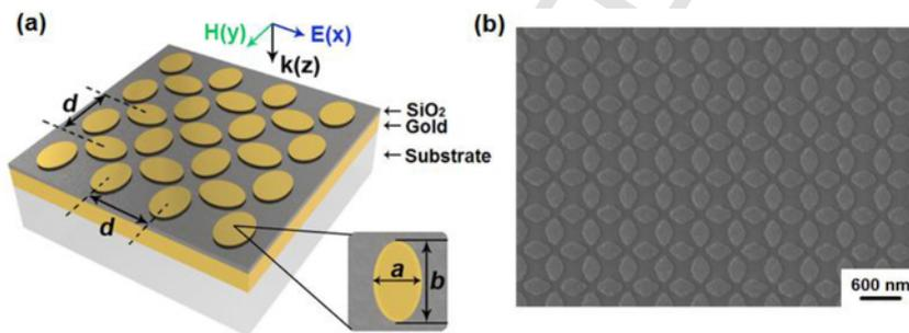
Fig. 2. (a) Schematic of the dual-band perfect absorber structure and the incident polarization configuration. (b) A SEM image of the designed structure. @OSA (extracted with permission from ref 8 - <https://doi.org/10.1364/OE.19.015221>).
