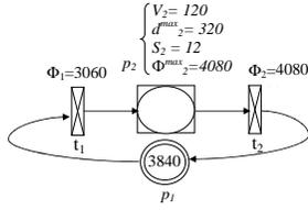
Fig. 6. CTBPN model of road section  $S$
