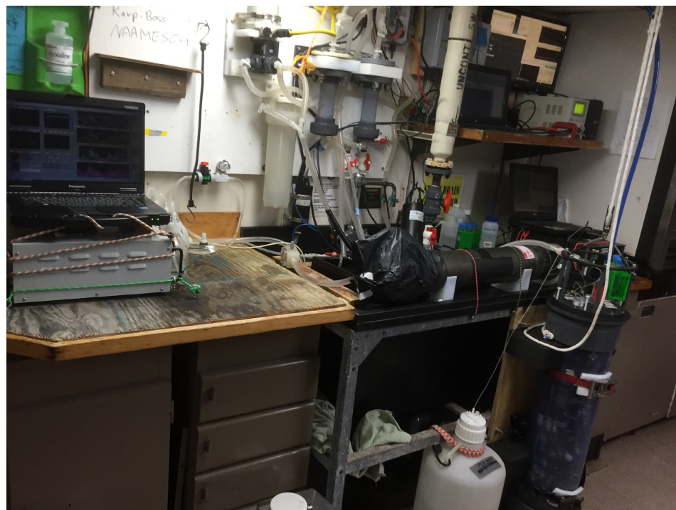
An example of a flow-through system that could be incorporated on GO-SHIP cruises as one component to study plankton. It includes an automated microscope to capture the community of chlorophyll containing particles (McLane's IFCB), a spectro-fluorometer and fast-repetition-rate-fluorometer (WETLabs's ALFA) to study phytoplankton physiology, a particle sizer (Sequoia Scientific's LISST-100X) and a series of bio-optical instruments (WETLabs' AC-S, ECO-BB3, and CDOM fluorometer) to study the signature of upper-ocean plankton on the ocean color signals measured from space as well as constrain photosynthesis. Ocean water to this system is pumped with a diaphragm pump to minimize the impact on particles and is passed through a thermosalinograph (SeaBird's TSG) to provide environmental information. This system has been installed around a sink of the R/V Atlantis as part of the NASA-funded NAAMES project (Photo credit: Lee Karp-Boss).
