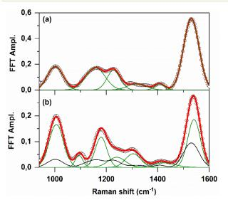
Figure 5: Multi-Gaussian fit of (a) DA and (b) LA non-resonant DFWM FFT spectra probed at 590 nm. The series of Gaussians represented by green curves in each graph. Black line in (b) represent the spectra of AT isomer which is kept constant during this constrained fit.
