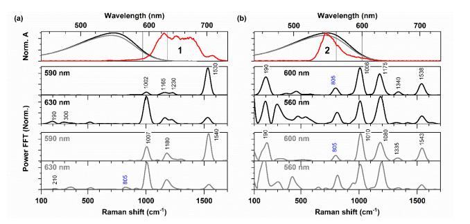
Figure 12: DFWM FFT spectra obtained by using near-resonant (1) and resonant (2) excitation spectra for DA (black) and LA (grey) ASR detected at different probing wavelengths shown by vertical grey line in (a) and (b).
