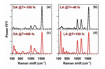
Figure 10: The relative amplification of low frequency modes probed at 590 nm before (black, T<0) and after (red, T>0) the arrival of actinic pulse for DA (a, c) and LA (b, d) ASR.
