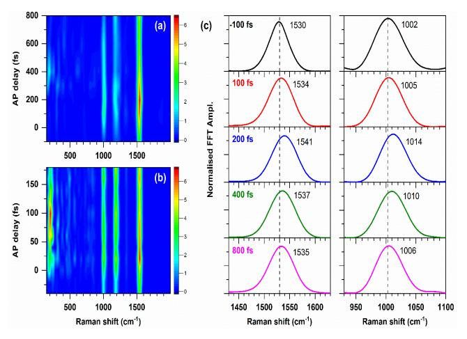
Figure 7: The evolution of pump-DFWM FFT spectra probed at 590 nm for (a) DA and (b) LA ASR with the actinic pulse delay. (c) The frequency shift of C=C stretch (left) and CH<sub>3</sub> rocking (right) mode for DA ASR with different actinic pulse delay. The black dotted lines represent the central frequencies obtained for AT GS (Fig. 6). The frequency shifts of the corresponding modes in LA ASR are shown in Fig. S6 of ESI.
