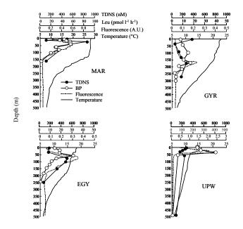
**Fig. 2.** Depth profiles of total dissolved neutral sugars (TDNS in nM), leucine incorporation rates (LEU, pmol  $1^{-1}$  h<sup>-1</sup>), chlorophyll fluorescence (arbitrary unit), and temperature (°C) at the four stations in the South East Pacific.
