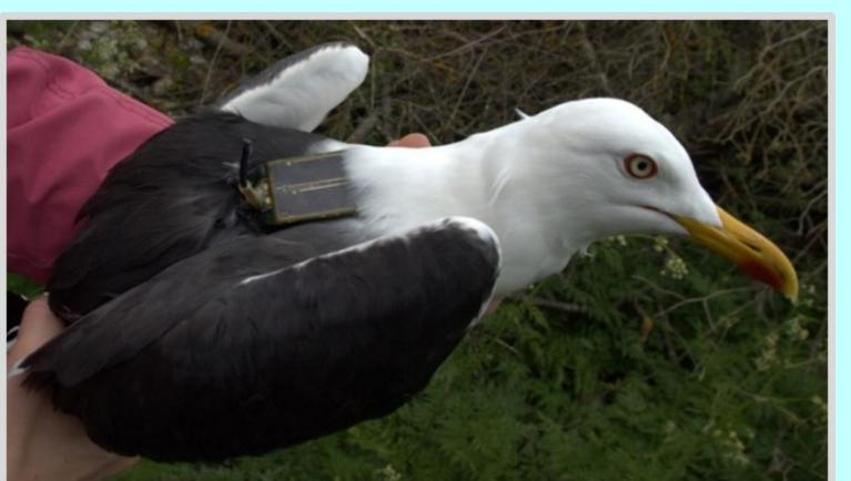
Lesser black-backed gull Larus fuscus equipped with Bio-logger UvA-BiTS (Sampling interval of the GPS: 15 sec)
