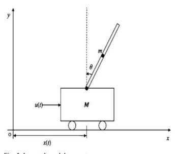
Fig. 5. Inverted pendulum system.
