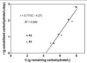
**Fig. 3** Rate of total carbohydrate solubilization *r* (g solubilized carbohydrate/L/day) vs. concentration of unutilized carbohydrate C (g remaining carbohydrate/L). Mean of steady-state solubilization data of each residence time (RT) of R2 and R3 (shown in Additional file 4: Table S3) was used to calculate *C* and *r*. Linear regression was performed and fitting curve was shown as solid black line in the figure
