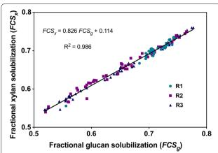
**Fig. 2** Comparative solubilization of xylan and glucan. Data are for the same samples reported in Fig. 1. Best fit linear regression curve is shown as solid black line
