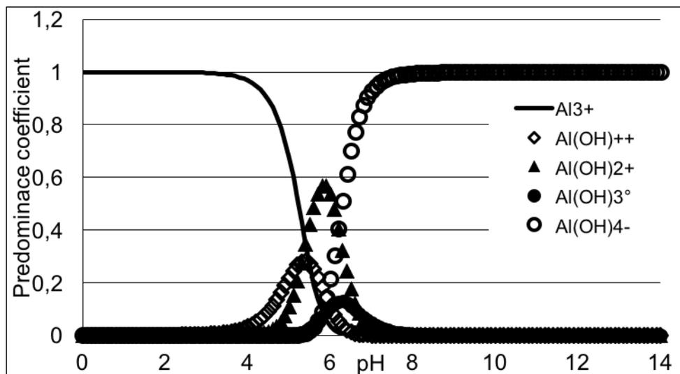
Figure 4: Species predominance diagram of aluminum in water at NaCl concentration = 0.150 mol.L<sup>-1</sup>
