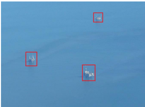
Fig 2: The detected platforms using Haralick features.
