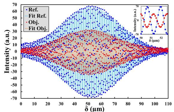
**Fig. 2.** Interference traces obtained on the same iso-phase curve in a reference point unmodified by the nanosecond laser beam during the grating inscription (in blue) and one in the center of a line composing the grating (in red). The inset is a magnification at the center of the traces.
