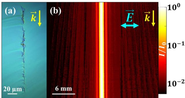
**Fig. 5.** (a) NIC micrograph of a cross section of one line composing a grating of period  $\Lambda = 100 \mu\text{m}$  written at  $0.5 \text{ mm/s}$ . (b) Diffraction pattern of the corresponding grating. The vector  $\vec{k}$  shows the direction of propagation.
