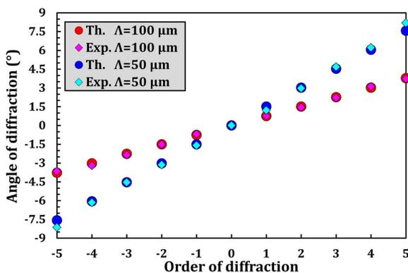
**Fig. 3.** Comparison between the theoretical values (circles) of the angle of diffraction for the different orders according to Eq. (1) and experimental measurements (squares) for gratings of period  $\Lambda = 100$  (red) and  $50 \mu\text{m}$  (blue).
