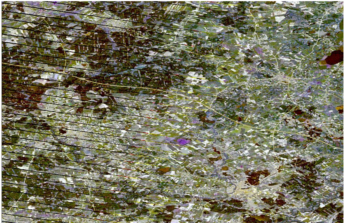
Figure 1: Example of geometric distortions on Landsat 7 ETM+ data
