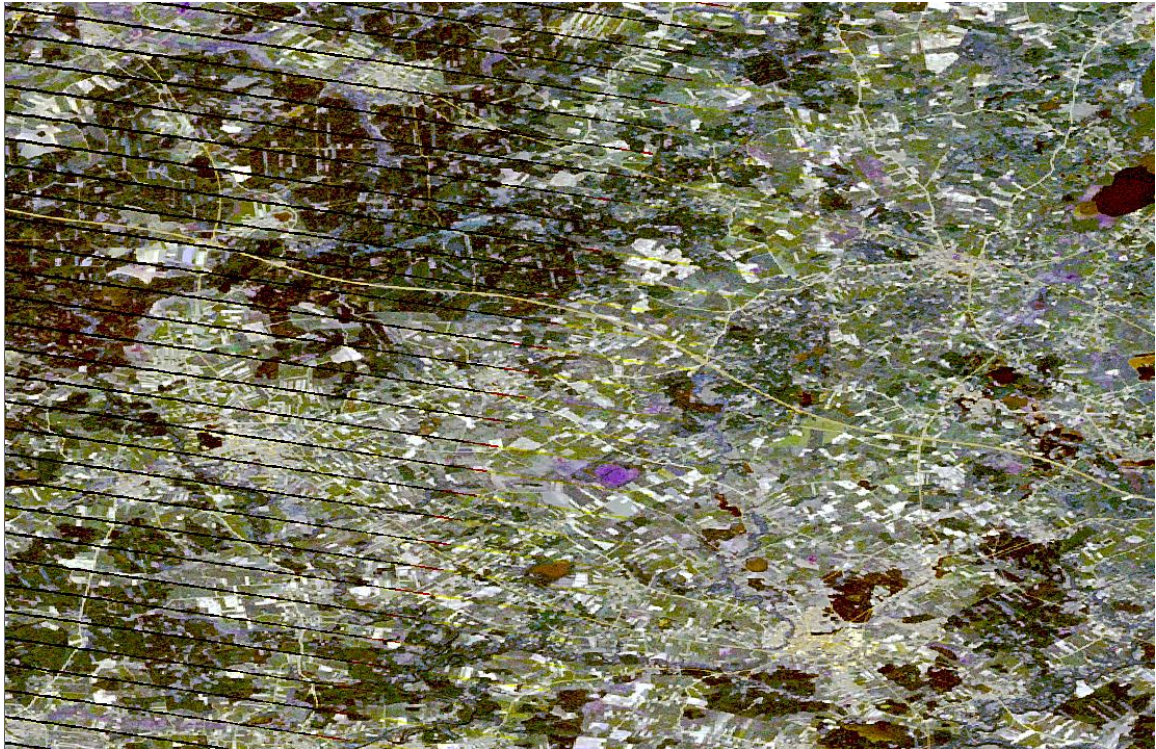
Legend: Landsat 7 ETM+, Klaipeda region, 01/05/2012, Recognition of Urban areas and road infrastructures (gold) by ensemble operator, missing information (black stripes) Sébastien Gadal, 2012.
