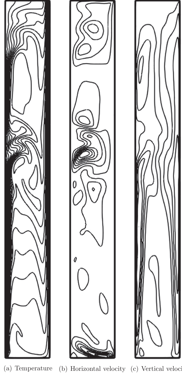
Fig. 9. Contours of temperature, velocities on 200 \times 1600 grid obtained by the present LB model for natural convection in a tall enclosure with a large temperature difference of \epsilon = 0.8 .
