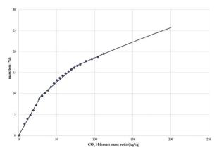
Fig. 7. JC SC-CO<sub>2</sub> extraction curve published by Micic et al. and modelled with BIC model (extraction of type B, P = 30 MPa and T = 323 K).
