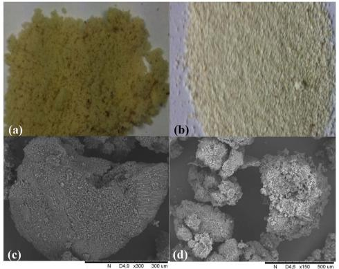
Fig. 3. grinded and sieved JC kernels (a) before extraction, (b) after extraction, (c) & (D) SEM before extraction.
