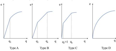
Fig. 1. Shapes of the extraction curves for the different types of extraction reported in the Sovová's mathematical model.
