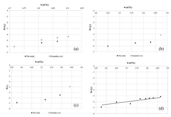
Fig. 6. JC oil solubility in SC-CO<sub>2</sub>, plot of  $\ln(y_s)$  versus  $\ln(\rho_{CO2})$ : (a) 313 K, (b) 323 K, (c) 333 K, (d) Chrastil modelling at pressure from 20 up to 40 MPa and temperature from 313 up to 333 K.
