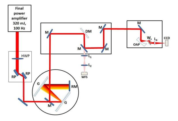
**Fig. 4** Experimental set-up for high-intensity experiments. It is made of an energy attenuator, the compressor chamber, the adaptive optics chamber and the interaction chamber. The propagation of the laser beam is represented by the red line. *HWP* half-waveplate, *RP* Brewster cut reflective polarizer, *G* diffraction grating, *RM* roof mirror, *M* dielectric coating mirror  $R_{\text{max}}$  in 750–850 nm spectral range, *DM*
