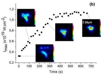
**Fig.7 a** Evolution of the differential beam wavefront measured at high energy (320 mJ per pulse) as compared with the wavefront measured at low energy (<30 mJ per pulse) after pre-compensation of the thermally induced wavefront distortions. **b** Evolution of the peak intensity delivered on target as a function of time. Snapshots of the beam profile in the focal plane are displayed to show the cor-
