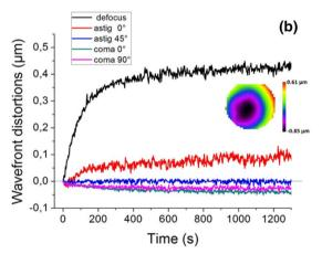
Fig. 5 Time-dependent evolution of the Zernike polynomial coefficients for an average power of 32 W before compressor (pulse energy of 320 mJ) with the deformable mirror (a) and with a dielectric
