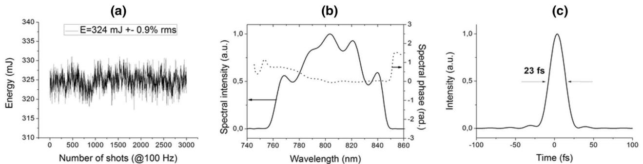
**Fig. 2** **a** Evolution of the pulse energy before compression. The average energy is  $\sim 324 \text{ mJ}$  per pulse with an energy stability of 0.9% rms. **b** Spectral intensity (solid lines) and phase (dot line) of the amplified
