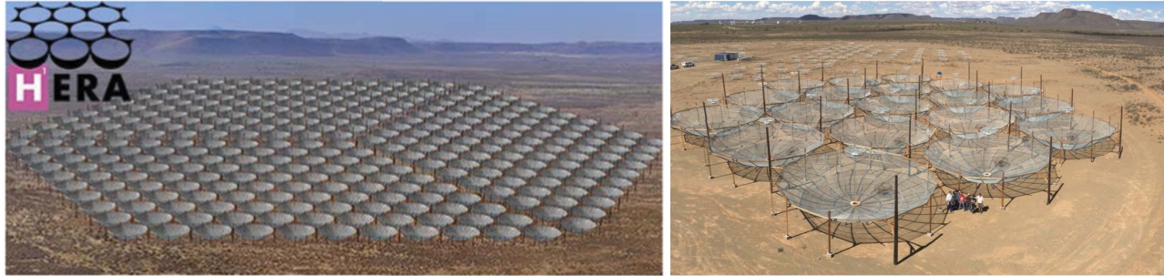
Figure 16. Left: Rendering of the 320-element core of the full HERA-350 array. Right: Picture of 19 HERA 14 m, zenith-pointing dishes (with PAPER elements in the background) currently deployed in South Africa. (Courtesy of James Aguirre)
