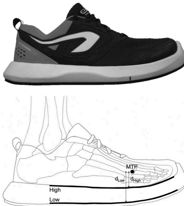
Figure 1. Picture of the shoe prototype used during the experiment (top), and locations of the stiff plate into the shoe (High and Low) with their respective distance ( d_{High} and d_{Low} ) from the metatarsophalangeal joint center of rotation (MTP) (down). Subtracting d_{High} from d_{Low} equaled the forefoot midsole thickness (12 mm).
