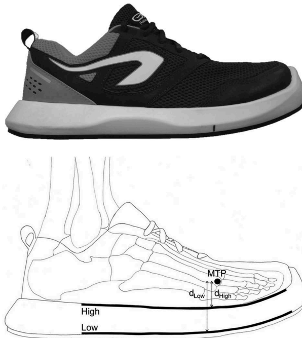
Figure 1. Picture of the shoe prototype used during the experiment (top), and locations of the stiff plate into the shoe (High and Low) with their respective distance ( d_{\text{High}} and d_{\text{Low}} ) from the metatarsophalangeal joint center of rotation (MTP) (down). Subtracting d_{\text{High}} from d_{\text{Low}} equaled the forefoot midsole thickness (12 mm).
