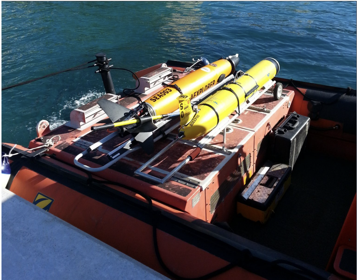
Figure 13. SOCIB and MIO glider units (Slocum and SeaExplorer, respectively) during the deployment.
