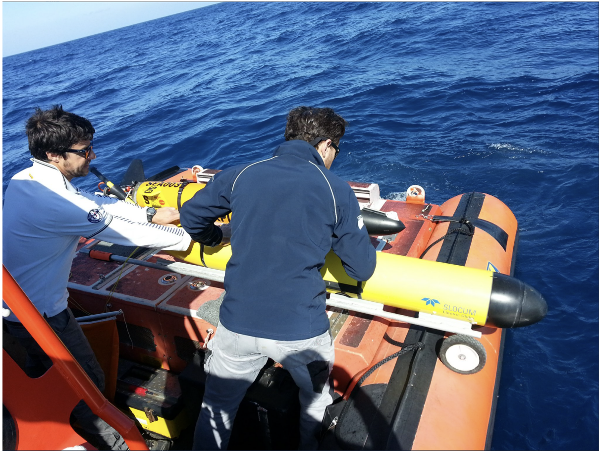
Figure 14. Deployment of the SOCIB Slocum glider.
