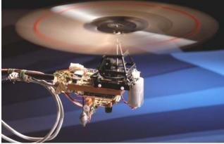
**Fig. 1.** The robot OCTAVE equipped with a ventral OF sensor and an *OF regulator* mimics insect behaviour in the vertical plane
