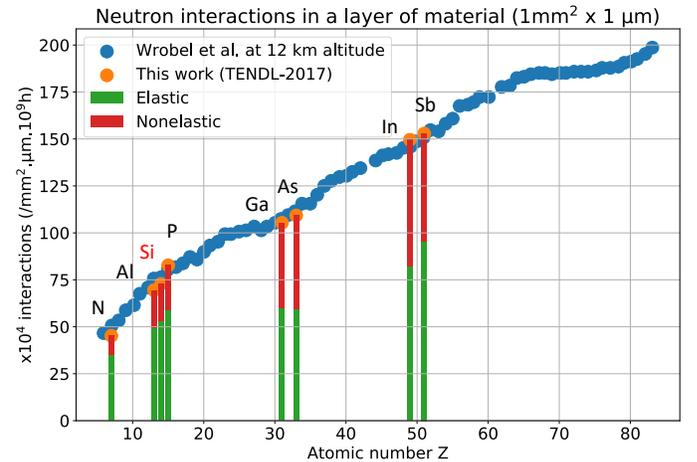
Fig. 3. Calculated number of nuclear interactions in  $10^9 \text{ h}$  induced by high energy (>1 MeV) atmospheric neutrons in a layer of material of  $1 \text{ mm}^2$ . Data are compared to previous results published in [16].
