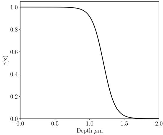
Figure 1. Depth distribution  $f(x)$  of created self-damaged traps.
