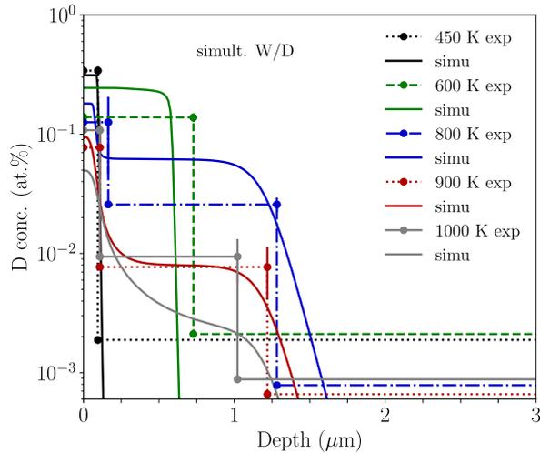
Figure 3. Comparison between the simulated and experimental D depth profiles after the simultaneous W/D exposure at the given temperatures during the experiments.
