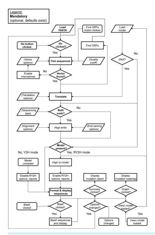
**Figure 1 Algorithmic flowchart of the implementation of 2HybridTools.** The flow of information is represented by arrows. Parallelograms represent inputs, rounded rectangles events, straight rectangles processing steps, and diamonds represent conditions. Fields in bold represent mandatory steps.
