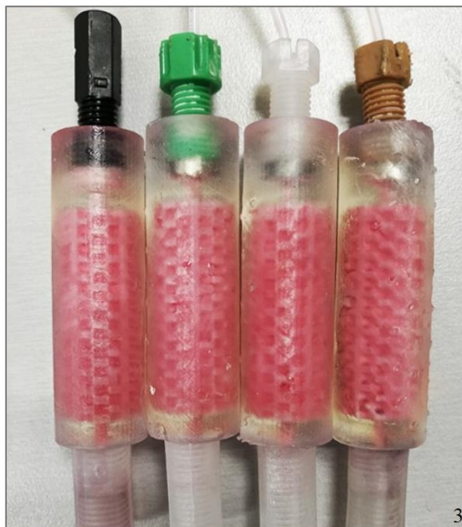
Figure S1: Pictures of 3D printed objects during grafting steps (1: raw resin disks; 2: grafted resin disks; 3: grafted cuboids columns).
