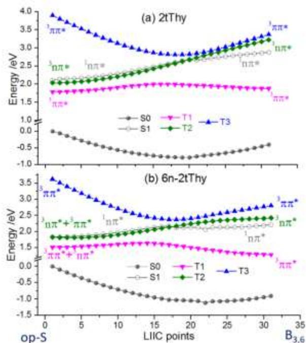
Figure 5 Potential energy profiles of the lowest singlet and triplet states and their characters for (a) 2tThy and (b) 6n-2tThy at CASPT2 level.
