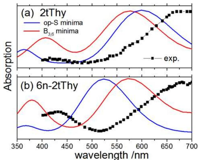
Figure 7. Experimental transient absorption spectra<sup>1</sup> at starting time and simulated absorption spectra from T<sub>1</sub> state for (a) 2tThy and (b) 6n-2tThy.
