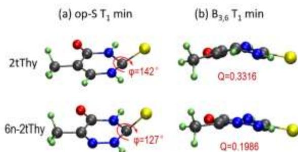
Figure 2  $T_1$  minima including (a) out-of-plane S (op-S) and (b) boat-distorted ( $B_{3,6}$ ) conformations of 2tThy and 6n-2tThy at CASPT2 level. In (a), the C/N6-N1-C2-S dihedral angle is indicated. In (b), the Cremer-Pople parameter Q, giving the ring puckering degree (in Å), is given as well. (Q = 0 corresponds to a planar structure.)
