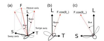
Fig. 1. (a) Resolution of the mean flight-force vector F along the surge X-axis giving the forward thrust T, along the sway Y-axis giving the side thrust S, and along the heave Z-axis giving the vertical lift L. (b) Pitching the mean flight-force vector F by an angle  $\theta_{pitch}$  generates a forward thrust T. (c) Rolling the mean flight-force vector F by an angle  $\theta_{roll}$  generates a side thrust S.
