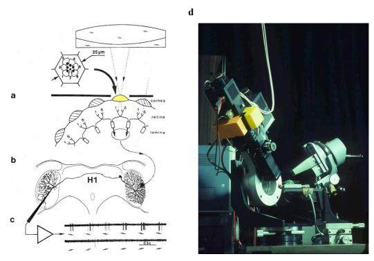
Fig. 2: (left): (a-c) Principle of the experiment aimed at deciphering the principle of motion detection in flies, using optical stimulation of single photoreceptors. (d) Triple-beam incident light "microscope-telescope" that *successively* delivers a 1µm light spot to two neighboring photoreceptor cells, R1 and R6, as shown in (a). A microelectrode records the electrical response of the motion sensitive neuron H1 to this "apparent motion" [27]
