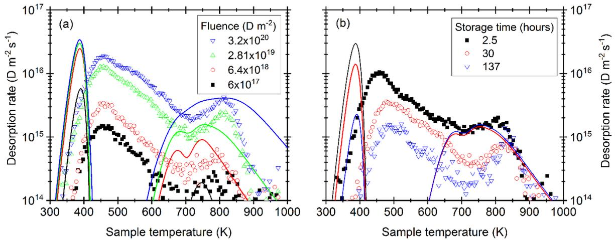
Figure 2. TPD measurements (symbols) on SCW performed (a) 2.5 hours after four different implantation fluences, and (b) for three different storage times after an implantation of  $2.81 \times 10^{19} D^+ m^{-2}$  at room temperature. Lines are results of Model 3.
