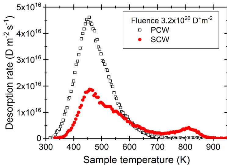
Figure 1. TPD measurements of deuterium desorption from single-crystal (SCW) and poly-crystals (PCW) tungsten samples after implantation of  $3.2 \times 10^{20} \text{ D}^+ \text{ m}^{-2}$  and a 2.5 hours storage time at 300 K.
