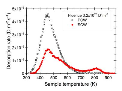
Figure 1. TPD measurements of deuterium desorption from single-crystal (SCW) and poly-crystals (PCW) tungsten samples after implantation of  $3.2 \times 10^{20}$  D<sup>+</sup>m<sup>-2</sup> and a 2.5 hours storage time at 300 K.
