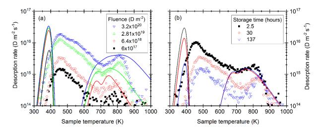
Figure 2. TPD measurements (symbols) on SCW performed (a) 2.5 hours after four different implantation fluences, and (b) for three different storage times after an implantation of  $2.81 \times 10^{19}$   $D^+m^{-2}$  at room temperature. Lines are results of Model 3.
