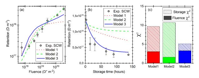
Figure 4. Three different MHIMS-R models compared to experimental results on SCW for (a) the deuterium retention as a function of fluence and (b) the dynamic retention of deuterium. Circles represent experimental data while lines are models results. (c) Pearson's chi-squared test obtained by comparing experimental and modeling results.
