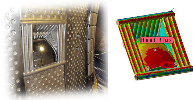
Fig. 3. Left: Mirror mounted in the inner wall of WEST - Right: calculated heat flux deposition pattern from plasma radiation (max = 130 kW/m 2 ).
