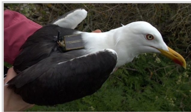
Figure 3. Lesser black-backed gull ( Larus fuscus ) equipped with an 18 g solar-powered UvA-BiTS device (size: 61×25×10 mm). The GPS unit used is the Lea-4S chip from U-blox manufacturer. See [9] for UvA-BiTS detail. Photographic credit: the authors.
