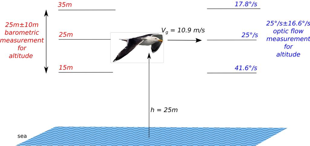
**Figure 9.** Altitude sensing in seabirds either by barometric pressure measurement or optic flow measurement at an altitude of 25m and a groundspeed of 10.9m/s generating a ventral optic flow of 25°/s.
