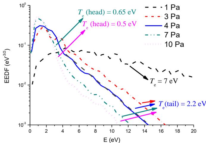
**Figure 4.** EEDF and the deduced electron temperatures as function of pressure at power of 400 W for 1 Pa and 1000 W for the higher pressure conditions. The temperatures are obtained assuming a Maxwellian or bi-Maxwellian distribution.
