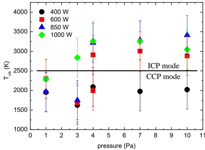
**Figure 10.** Vibrational temperatures of ground state  $H_2(X^1\Sigma_g^+, v)$  as a function of gas pressure for various delivered powers. The samples temperature was held at 300 K (without Pyrex tube). The vibrational temperatures are constant with pressure and power but differ markedly between the two discharge modes.
