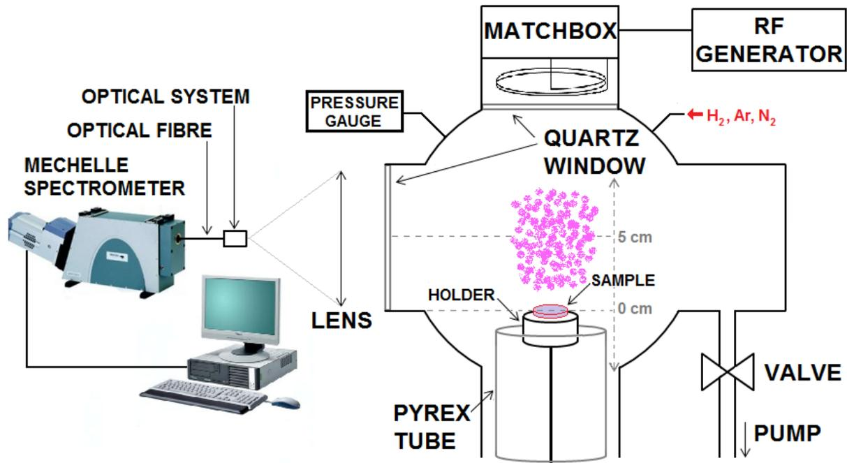
**Figure 1.** Illustration of the experimental set-up.
