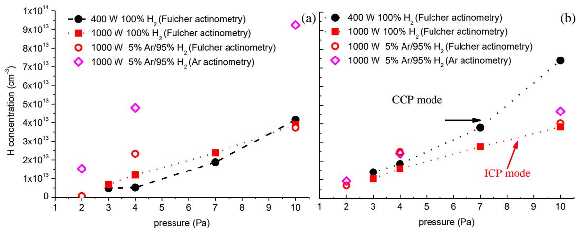
**Figure 12.** Evolution of atomic hydrogen concentrations with pressure at 400 and 1000 W while the sample holder temperature was held at 300K (without sample). On graphs (a) and (b) we are presenting the results of actinometric technique using the H-alpha and H-beta lines, respectively. The Fulcher- $\alpha$  and argon actinometry with H-beta line are in good agreement, the use of H-alpha should be avoided. The resulted H atom concentration is increasing with the pressure.
