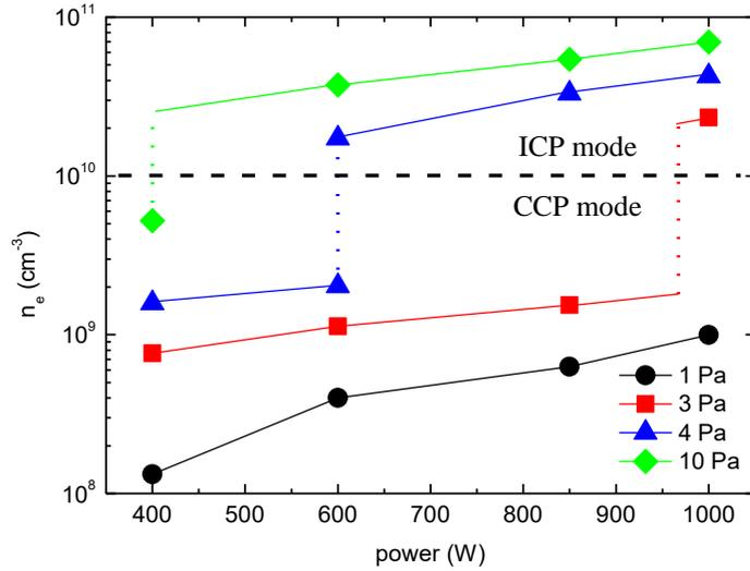
**Figure 2.** Electron density in pure H<sub>2</sub> plasma as function of pressure for powers between 400 and 1000 W. Overall, the electron densities are increasing by increasing power. The transition from CCP to ICP discharge mode is marked with dashed line. With increasing pressure this transition occurs at lower values of power.
