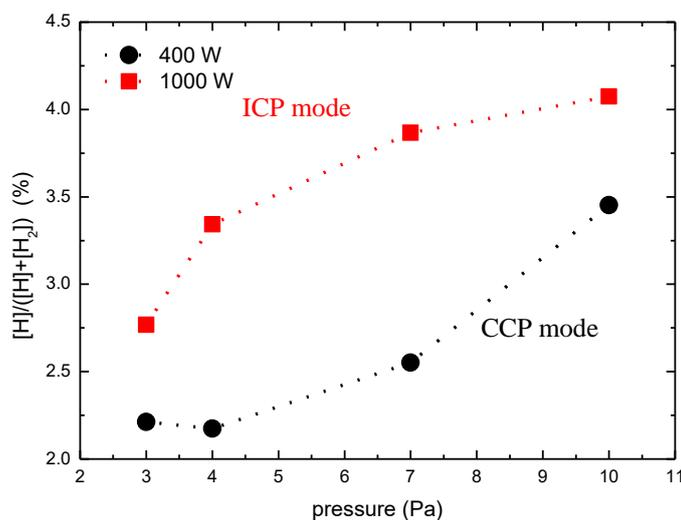
**Figure 13.** Dissociation ratio as function of pressure at 400 and 1000 W. The dissociation ratio is higher in the ICP mode than CCP mode.
