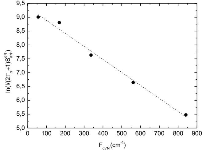
**Figure 5.** Boltzmann plot of rotational states for the vibrational transition  $\nu' - \nu'' = 1-1$  of the Q-branch of the Fulcher- $\alpha$  band (pure  $\text{H}_2$ , 4 Pa, 1000 W).
