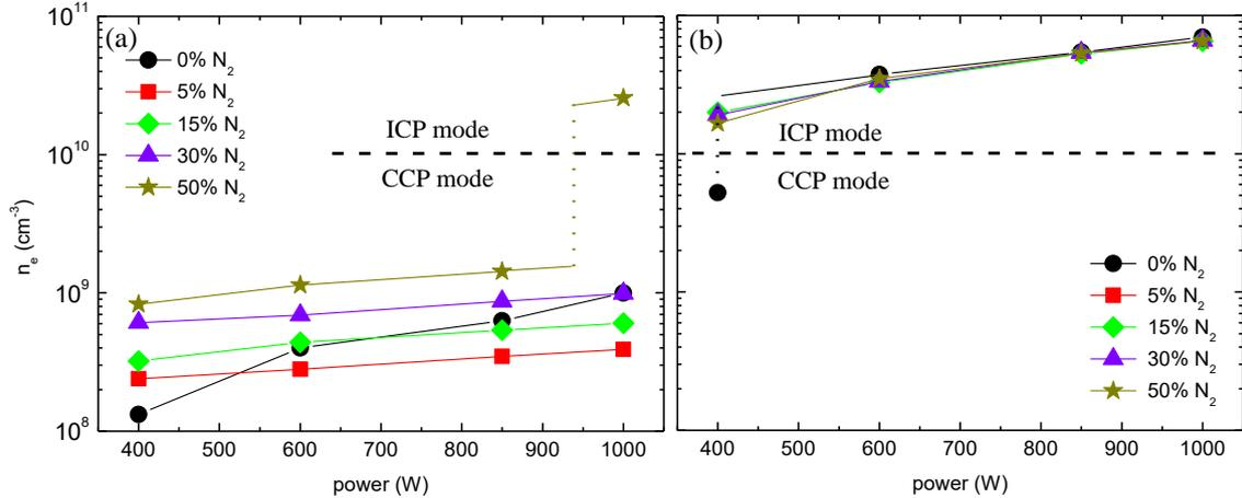
**Figure 3.** Electron density in mixture of H<sub>2</sub>-N<sub>2</sub> at 1 Pa (a) and 10 Pa (b) as function of power for different N<sub>2</sub> percentages. The transition from CCP to ICP discharge mode is marked with dashed line. Nitrogen addition was realized to help determine the gas temperature, however this led to some changes in the electron concentration compared to the case of pure hydrogen.
