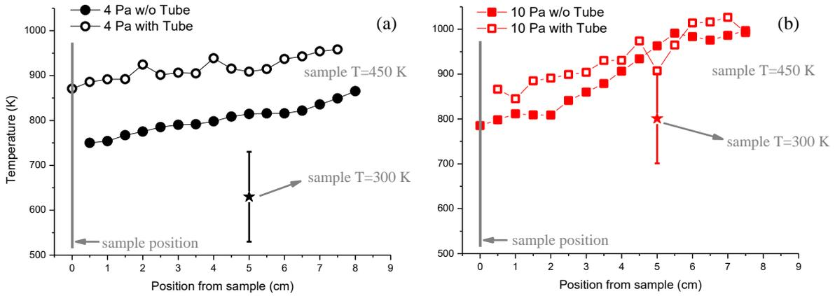
**Figure 8.** Evolution of gas temperature at 4 Pa (a) and 10 Pa (b) with (empty symbols) and without Pyrex tube (full symbols). The points marked by stars are measured without Pyrex tube and heating of sample to 300 K. Other measurements are done at 450 K of sample holder. The Pyrex tube delimited the chamber and also the discharge to smaller dimensions, increasing the power density resulting in higher temperatures of the gas.
