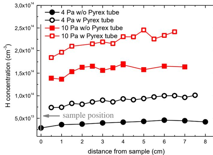
**Figure 14.** Evolution of atomic hydrogen concentration at 4 Pa (black colour) and at 10 Pa (red colour) with Pyrex tube (empty circle) and without Pyrex tube (full circle) at power of 1000 W and temperature of sample holder 450 K. The gas mixture was H<sub>2</sub> / 5 % Ar. H-beta line has been used. The H atom concentration is higher with the tube due to higher power density and the choice of wall material, as Pyrex is reducing atomic loss.
