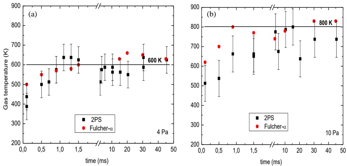
**Figure 7.** Evolution of gas temperature during one pulse (ON:OFF = 50ms:50ms) at 1000 W in 50 % nitrogen admixture at pressures of 4 (a) and 10 Pa (b). Black line shows gas temperature in the case of the continuous discharge. The temperature is increasing during the pulse and reaches a stationary value after  $\sim 1.5$  ms, which corresponds to the value of  $T_g$  in the continuous discharge.
