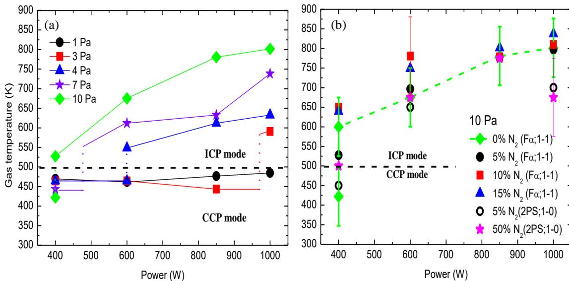
**Figure 6.** Gas temperature in pure hydrogen as function of pressure determined from Boltzmann plot of vibrational band 1-1 of Fulcher- $\alpha$  (a). Comparison of gas temperatures at 10 Pa as function of delivered power in the case of nitrogen admixtures determined from vibrational band 1-1 of Fulcher- $\alpha$  for 0, 5, 10 and 15 %  $N_2$  (full
