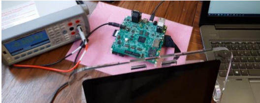
Figure 3: View of the test installation with the development board in the middle connected to the monitoring PC.
