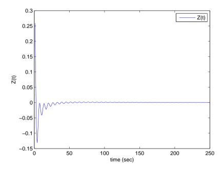
Figure 1. Response of the controlled output z(t)
