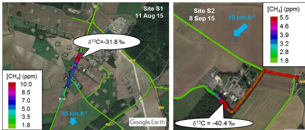
Figure 5. Left : Methane concentration measured by CRDS on 11 Aug. 2015 at Gournay-sur-Aronde (site S5) showing a local methane enhancement of 8.1 ppm above background concentration with a \delta^{13}\text{CH}_4 signature of -31.8 \pm 2.0 \text{ ‰} . Right : Same but at Germigny-sous-Coulombs on 8 September 2015 at Germigny-sous-Colombs (site S2) showing a local methane enhancement of 3.5 ppm above background with a \delta^{13}\text{CH}_4 signature of -40.4 \pm 2.0 \text{ ‰} (CRDS, 8 September 2015). The blue arrow and label indicate wind direction and speed. The color scale is automatically adapted to each survey by the Picarro investigator unit software.
