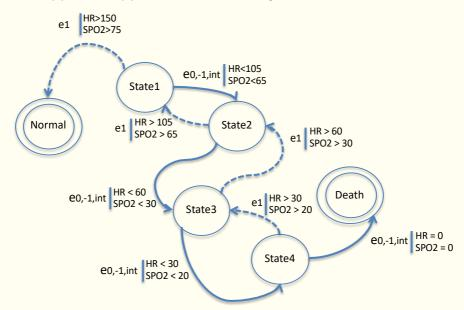
**Figure 11**: State-chart diagram modelling the new-born's behaviour according to the right or wrong execution of the ventilation gesture.  $e_{0,-1,int}$  is a shortened notation meaning that the degradation transition can be  $e_0$ ,  $e_{-1}$ , or  $e_{int}$ .
