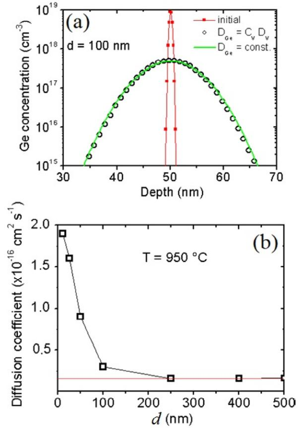
**Fig. 3.** Simulation results of Ge diffusion in a 1D Si nanocrystal using Eqs. (1) and (2): a) Ge concentration profiles in a 100 nm-thick 1D crystal, the red solid squares, the open solid circles, and the green solid line correspond to the initial Ge profile, the Ge profile after annealing at 950 °C for one hour, and the numerical fit of the Ge profile after diffusion using Eq. (3), respectively; b) variations of the Ge effective diffusion coefficient versus the nanocrystal size  $d$ .
