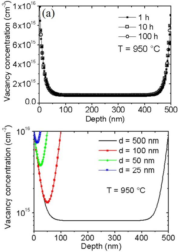
**Fig. 2.** Vacancy concentration profiles simulated at  $T_a = 950\text{ °C}$  using Eq. (1): a) versus annealing time in a 500 nm-thick 1D crystal; and 2) versus the 1D nanocrystal size  $d$  after one hour annealing.
