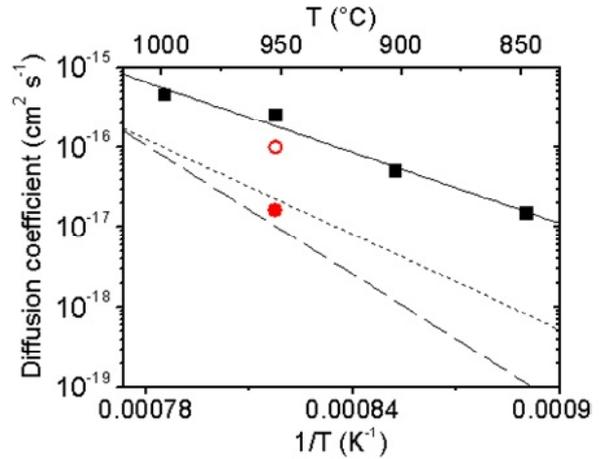
**Fig. 4.** Ge diffusion coefficients measured in the Si mono-crystal (dot line from [31] and dash line from [32]) and in  $40 \text{ nm}$ -wide Si grains (solid square [14]), compared with the corresponding coefficients obtained in the simulations at  $T = 950 \text{ }^\circ\text{C}$  (red solid circle in the mono-crystal and red open circle in the nano-grain).
