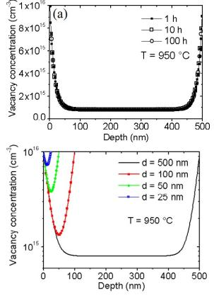
Fig. 2. Vacancy concentration profiles simulated at  $T_a = 950$  °C using Eq. (1): a) versus annealing time in a 500 nm-thick 1D crystal; and 2) versus the 1D nanocrystal size d after one hour annealing.
