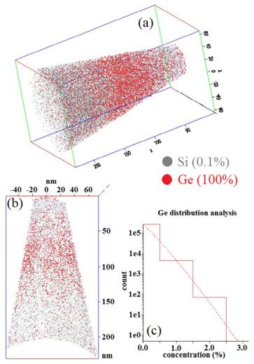
**Fig. 1.** APT measurements performed on the Ge-implanted Si nanocrystalline layer annealed at 850 °C for one hour: a) an entire APT volume showing 0.1% of the detected Si atoms (gray dots) and 100% of the detected Ge atoms (red dots); b) a 20 nm-thick slice taken in the center of the same volume; and c) the atomic distribution of Ge atoms in the APT volume (solid line) compared to an atomic random distribution (dash line).
