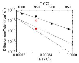
**Fig. 4.** Ge diffusion coefficients measured in the Si mono-crystal (dot line from [31] and dash line from [32]) and in 40 nm-wide Si grains (solid square [14]), compared with the corresponding coefficients obtained in the simulations at T = 950 °C (red solid circle in the mono-crystal and red open circle in the nano-grain).
