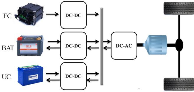
Fig. 1: Vehicle configuration.
