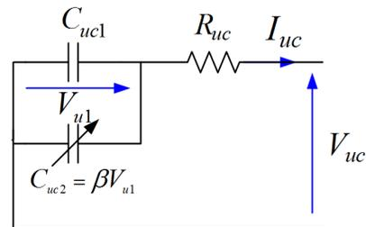
Fig. 5: Ultracapacitor model
