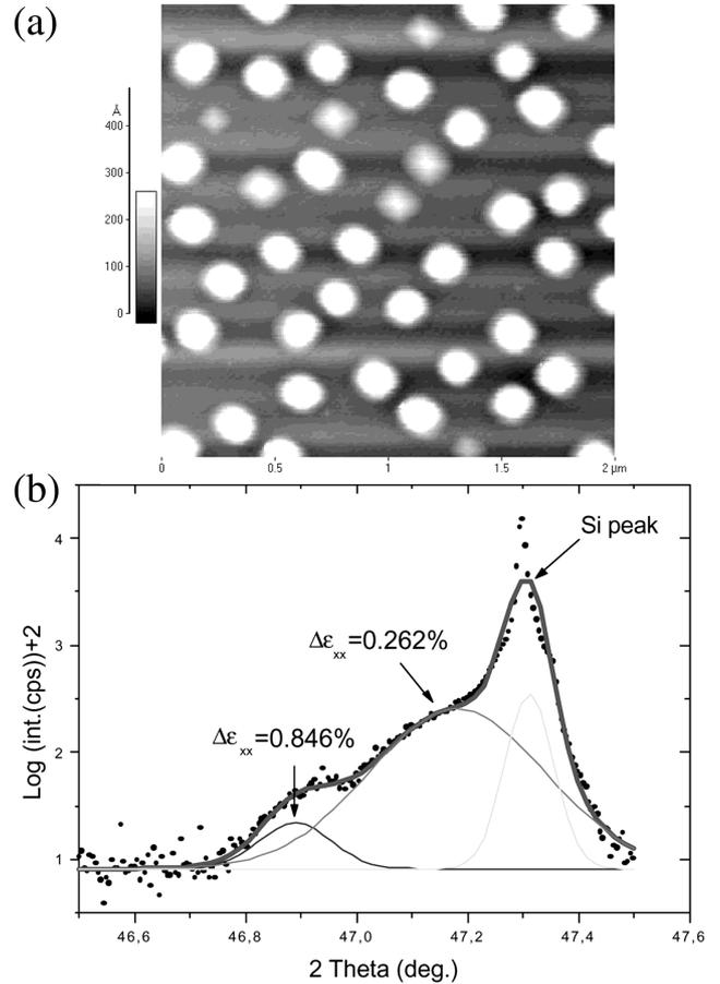
Fig. 8. (a) AFM image and (b) GIXRD spectrum of ‘hut’ and ‘domes’ stabilised during the h annealing at 550°C of a  $\text{Si}_{0.6}\text{Ge}_{0.4}$  ( $h = 5$  nm). Elastic relaxation of  $\Delta\varepsilon_{xx} \sim 0.85\%$  and  $\Delta\varepsilon_{xx} = 0.25\%$  were estimated for ‘domes’ and ‘huts’ respectively.
